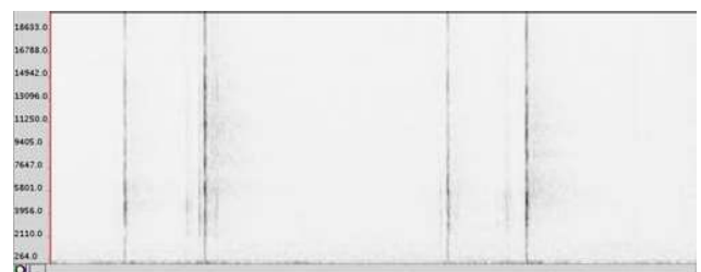
Figure 5: Clicks of a ball-pen. Time-frequency resolution: b_{crit} = 196.53Hz . This sound has mainly transient components with very temporal characteristics.
