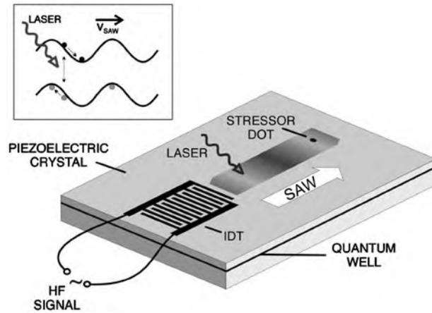
**Figure 21.** A schematic illustration of acoustically pumped quantum dots showing a quantum well on a piezoelectric crystal (for example, an InGaAs QW on a GaAs substrate) and a stressor dot which may be formed e.g. by InP. Laser-excited excitons in the quantum well are dissociated by high-frequency piezoelectric fields produced by the SAW. The released electrons and holes are then stored in the moving potential of the SAW, as shown in the inset (after Wiele *et al* (1998)).
