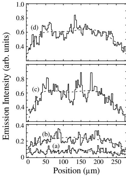
**Figure 8.** Evolution of the emission intensity cross section with driving amplitude at a given location on the illuminated surface (figure 1) of more packed ZnS:Mn grains ( $\eta \approx 0.43$ ). Panels (a), (b), (c) and (d) are taken at  $U$  denoted by arrows a, b, c and d, respectively in figure 10 (closed circles). After Korotchenkov and Goto (1999).
