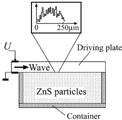
**Figure 1.** A schematic side view of the acoustic cell used for the observation of acoustically induced luminescence in ZnS grain mixtures. The rf driving voltage  $U$  in the MHz range is applied to the  $\text{LiNbO}_3$  piezoelectric plate. The container confines ZnS particles in a mm-sized bed. The light emission discussed in section 2.2 is imaged in a  $0\text{--}250\ \mu\text{m}$  illuminating spot.
