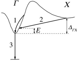
**Figure 5.** A schematic diagram of the transitions within the  $\Gamma$  and X valleys in the band structure (1 and 2) as well as defect-related radiative recombination (3) used to explain the spectra of acoustically induced luminescence in ZnS powders.
