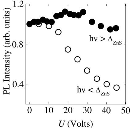
**Figure 15.** Time-integrated PL intensities of the 5 ML QW versus driving amplitude. The PL has been excited by photon energies of 4.0 eV (closed circles) and 3.5 eV (open circles), respectively (Korotchenkov *et al* 1999).
