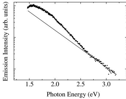
**Figure 6.** The wavelength dependence of the measured emission spectrum for ZnS:Mn grains from figure 2 on a semilog scale (circles) and the exponential fit (line) to the higher-energy side of the spectrum.
