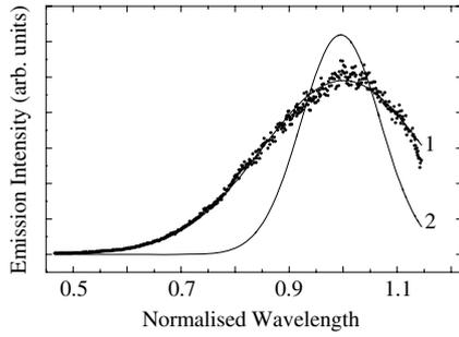
**Figure 4.** The wavelength dependence of the measured emission spectrum in ZnS:Mn grains from figure 2 (circles) and the best-fitting spectra obtained by using equation (2.5) (lines) for  $\delta = 0.2 \mu\text{m}$ ,  $\bar{r} = 1.5 \mu\text{m}$  (curve 1) and  $\delta = 0.11 \mu\text{m}$ ,  $\bar{r} = 1.5 \mu\text{m}$  (curve 2). The wavelength is normalized to the maximum position of the measured spectrum.
