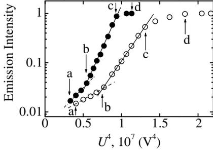
**Figure 10.** Logarithm of emission intensity  $I$  as a function of  $U^4$ . Solid and dashed lines indicate fits to equation (2.16) by using data points at which they intersect (after Korotchenkov and Goto (1999)).
