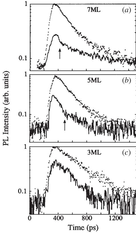
**Figure 17.** Transient PL intensities from QWs at photon energies 3.052, 3.097 and 3.138 eV for the 7 ML (a), 5 ML (b) and 3 ML (c) wells, respectively, after picosecond excitation at 4.0 eV at  $t \approx 200$  ps. The dotted and solid curves correspond to  $U = 0$  and 45 V, respectively. After Korotchenkov *et al* (1999).
