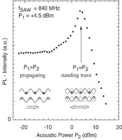
**Figure 19.** PL intensity as a function of the acoustic power  $P_2$  from IDT<sub>2</sub> for a constant acoustic power  $P_1 = +5.5$  dB m. The insets illustrate the storage of excitons in the SAW potential. The frequency of the SAWs  $f_{\text{SAW}1} = f_{\text{SAW}2} = 840$  MHz (after Rocke *et al* (1997)).
