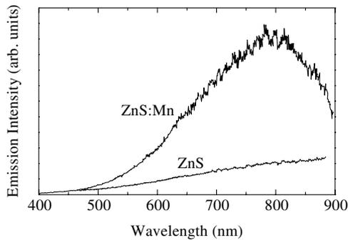
**Figure 2.** Spectra of acoustically induced luminescence from ZnS:Mn and ZnS grains (Korotchenkov and Goto 1997). Using a driving voltage of  $U \approx 70$  V, the total radiance is roughly  $10^{-13}$  W and  $0.2 \times 10^{-13}$  W in doped and undoped mixtures, respectively.
