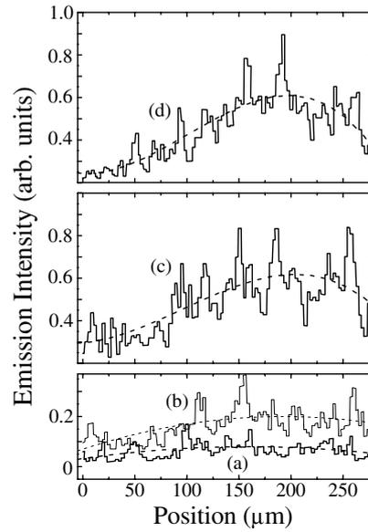
**Figure 9.** The same evolution as in figure 8, but with the grain mixture prepared under less packed initial conditions ( $\eta \approx 0.37$ ). Panels (a), (b), (c) and (d) are taken at  $U$  denoted by arrows a, b, c and d, respectively (open circles), in figure 10. After Korotchenkov and Goto (1999).
