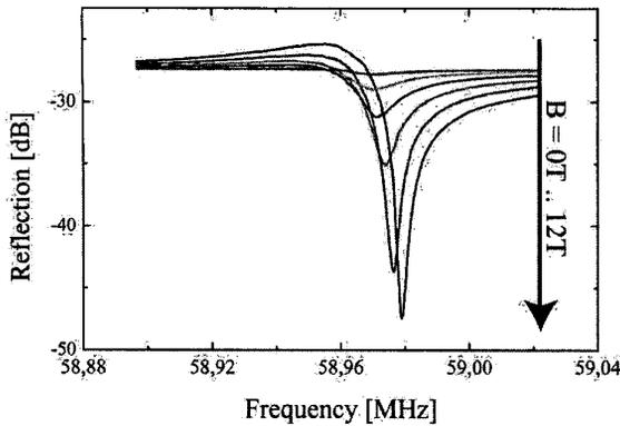
**Figure 3. Measured resonance at 59 MHz for increasing magnetic field, applying a power of -52 dBm. The quadratic dependence of peak height on magnetic field proves the mechanical character of the resonance.**
