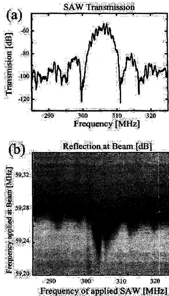
**Figure 6. (a) SAW transmission over the IDT delay-line.** The spectrum shows a typical  $\sin(f)/f$  dependence with a maximal SAW generation at 305 MHz (b) SAW induced changes in the resonance of the beam. The observed shifts corresponds to the SAW generation seen in (a).
