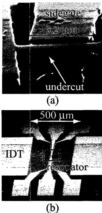
**Figure 1. (a) Close-up view of a beam resonator with 3.2 μm length, 300 nm height, and 500 nm width. Close to the freely suspended beam a sidegate is placed. The beam including mechanical supports was matched to a SAW wavelength of 9.2 μm (b) Sample's geometry showing the resonator placed in the path of two interdigitated transducers (ITD) for SAW generation.**
