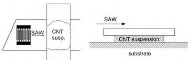
**Figure 2.** Sketch of the alignment setup. The SWNT suspension is placed in the capillary gap on the LiNbO<sub>3</sub> substrate, and a SAW is launched by the use of an interdigital transducer.
