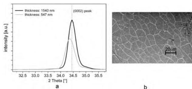
**Figure 4** (a) XRD pattern of two ZnO layers produced on Si (100) by PLD with different thickness. The XRD peak of the thinner film is shifted left because of high stress. XRD peak of the thick layer is relaxed, because of a break up of the layer (b) SEM pictures of the thick sputtered ZnO layer.
