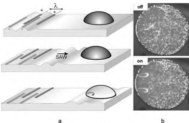
**Figure 5** (a) Principle of a SAW propagation on a piezoelectric layer; (b) mixing of a droplet (1.0 mm diameter) on a sputtered piezoelectric ZnO layer. By applying an alternating voltage the droplet is stirred up.
