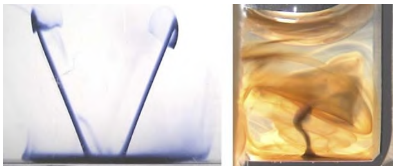
Figure 16.3 SAW induced fluid actuation in one of the wells in a microtiter plate (left) and in a quartz cuvette (right), visualized by the agitation of some ink initially located at the bottom. In the microwell, the IDT was placed directly under the well and has been coupled through its bottom. In this case, as the IDT is completely symmetric, two jets are excited under the Rayleigh angle \theta_R (Advantix AG, unpublished).
