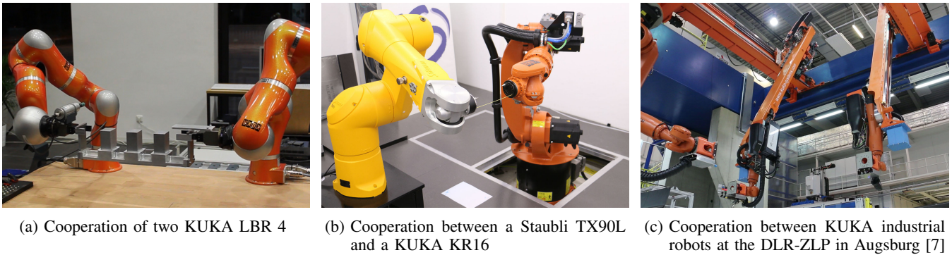
Fig. 4: Examples for cooperating industrial robots which are currently supported by the Robotics API.
