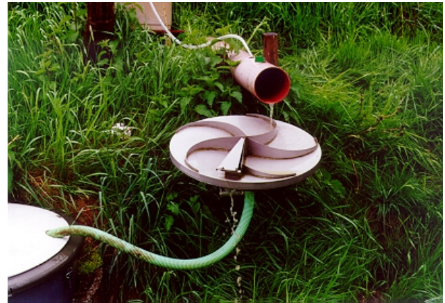
Figure 3. Coshocton-type wheel surface runoff sampling device and collecting tank used to monitor surface runoff and sediment delivery at all watershed outlets.
