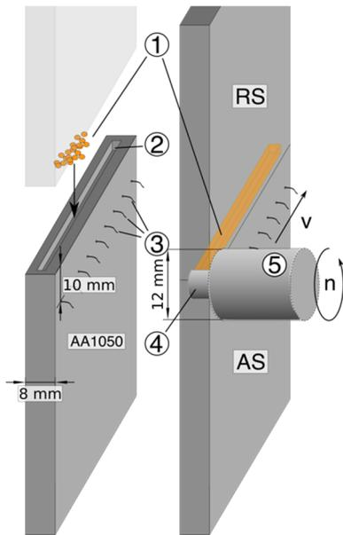
**Figure 1.** Schematic diagram of the sample production by a combination of Friction Stir Welding and Friction Stir Processing of the joint of two aluminium sheets with copper powder (1) in between. A groove (2) in the lower sheet is filled with commercially pure copper and the temperature during the process is measured by thermocouples (3). A rotating steel probe (4) with a shoulder (5) distributes the additional copper within the Aluminium matrix.
