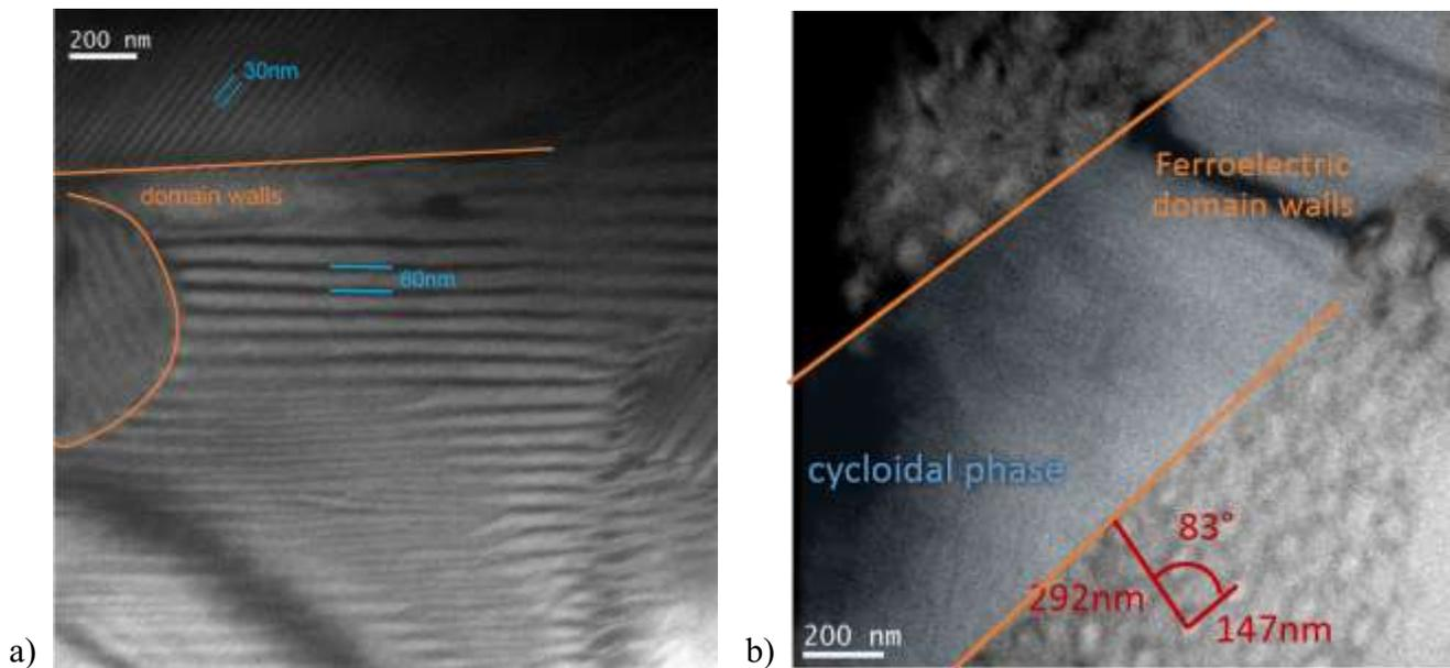
**Figure 1.** a) Cycloidal phase of GaV<sub>4</sub>Se<sub>8</sub> cut in <111> direction at 10K and 160mT: different sizes of the cycloidal phase are clearly visible; b) ferroelectric domains in GaV<sub>4</sub>Se<sub>8</sub> cut in <110> direction: ferroelectric domain walls separate cycloidal and skyrmion phase from each other
