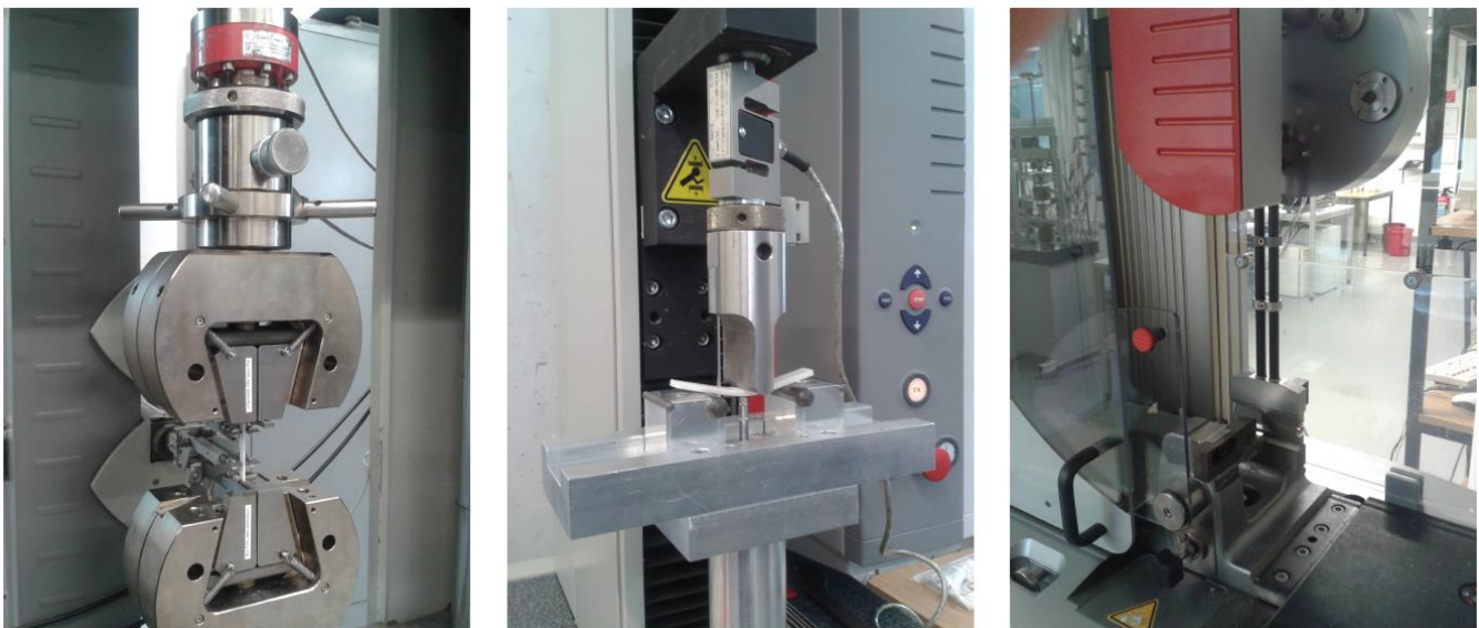
Figure 4 left: Tensile test with Zwick multiXtens extensometer. Middle: 3-point-bending test with linear inductive extensometer below the sample. Right: Impact test machine.
