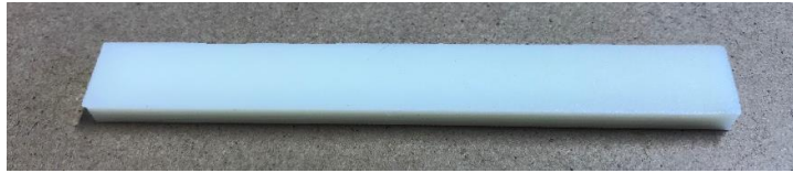
Figure 5: ABS sample produced by ARBURG freeformer
