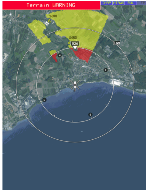
Figure 6.1.: Pilot interface of a helicopter application. Terrain that is higher than the current altitude is highlighted. The current position of the helicopter is displayed in the center of the picture. [52]
