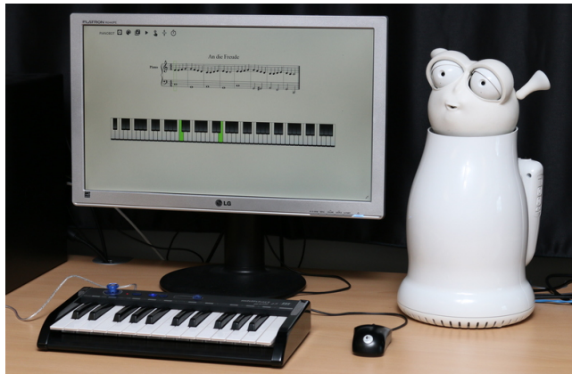
Figure 1: Hardware setup including a robot, a screen and a small MIDI keyboard.
