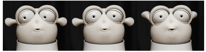
Figure 2: The robot’s gaze and facial expressions: a saccade (left), its neutral facial expression when centering on the spectator (middle) and smile (right).
