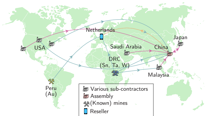
Figure I.1.: Supply chain of a contemporary electronic device at the example of a cell phone (“Fairphone 2”). Shown are known mines and pits for various raw materials, sub-contractors for individual parts like adhesives, integrated logic or glass. The assembly is in China, re-sellers in Europe. Drawn after reference [28].
