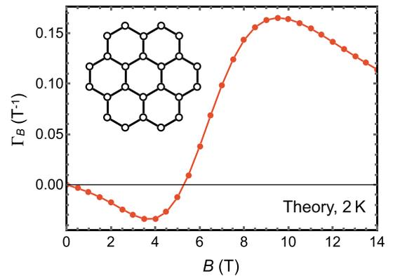
FIG. 3.  $T = 2$  K exact diagonalization results of the magnetic Grüneisen parameter  $\Gamma_B$  for the minimal model of  $\alpha$ -RuCl<sub>3</sub> [26]. The inset shows the employed periodic cluster.
