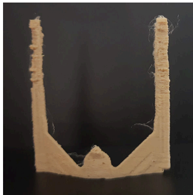
Fig. 1: A structure with two identical towers. During printing the tower base loosened from the print bed with the middle connecting structure remaining connected to the bed. The movement of the sides resulted in very inaccurate albeit finishing printing.
