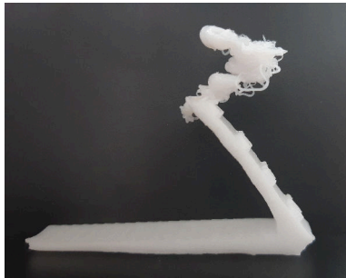
Fig. 2: A benchmark print that lost adhesion due to warping and then got dragged along until the human operator detected the issue. The warping is best visible to the lower left. The spaghetti print failure is visible to the top right where the print should have continued.
