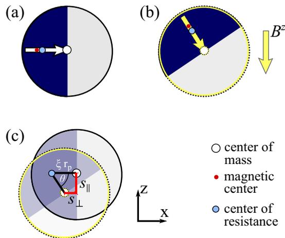
FIG. 7. Sketch of a sd particle (a) before (solid circle) and (b) after (dotted circle) rotation by  $\theta$  caused by  $B^z$ , and (c) an overlay of both situations considering that the particle rotates around the center of resistance that is shifted by  $\xi r_p$ . The center of the sphere moves by  $s_{\perp} = \sqrt{x^2 + y^2}$  ( $\perp B^z$ ) and  $s_{\parallel}$  ( $\parallel B^z$ ).
