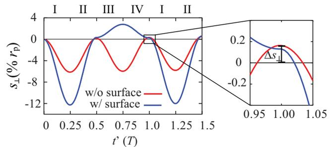
FIG. 10. Translations  $s_{\perp}$  of sd particles in a triple ring placed in a homogeneous environment (red curve) and close to a substrate wall (blue curve). The magnified inset on the right illustrates the overall distance a particle has traveled during one field cycle.
