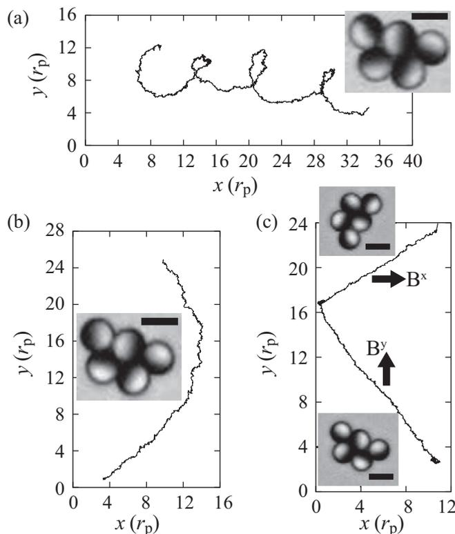
FIG. 2. Experimental trajectory of two compact clusters (insets) (a), (b) under an oscillating field with  $B^z = 0.53$  mT,  $\omega/2\pi = 5$  Hz (a: 88 s; b: 251 s) [42] and (c) under an oscillating field ( $B^z = 1.13$  mT,  $\omega/2\pi = 20$  Hz) and a constant in-plane field ( $B^{x,y} = 0.03$  mT) [43]. The in-plane field is switched from  $B^y$  to  $B^x$  during the recording (scale bars  $5 \mu\text{m}$ ).
