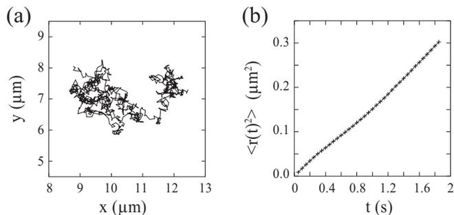
FIG. 8. Translational diffusion of a capped particle with a diameter of  $4.54 \times 10^{-6}$  m on a glass substrate while the rotational motion is suppressed by an external field. (a) Trajectory of a single particle moving on the  $xy$  substrate plane for a time sequence of 20 s. (b) Mean-squared displacement,  $\langle r(t)^2 \rangle$ , of the trajectory depicted in (a).
