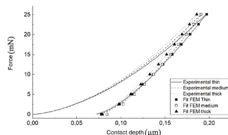
**Fig. 11** Force displacement curves measured normal to the coating surface (dotted lines) and best fit result from the FEM model for the measurement of coatings with different thicknesses deposited at the medium temperature.
