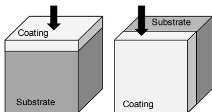
**Fig. 2** Schematic of the cross-sectional measurement (a) and the measurement normal to the coating surface (b).
