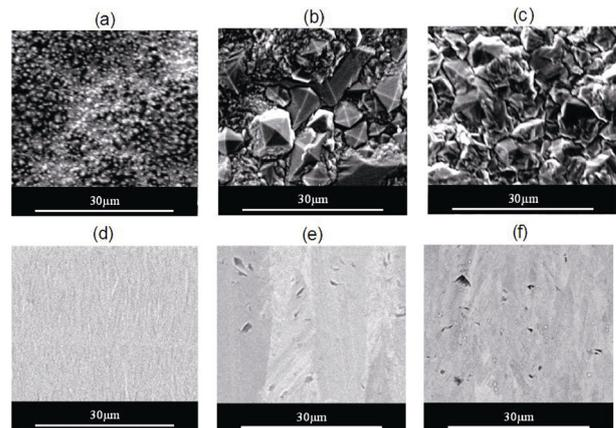
**Fig. 1** Surface scanning electron microscopy of silicon carbide coating with different deposition temperatures: (a) lowest, (b) medium, and (c) high; cross-sectional scanning electron microscopy images at different temperatures: (d) lowest, (e) medium, and (f) high.
