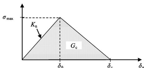
Fig. 8 Bilinear traction-separation law for the cohesive zone.
