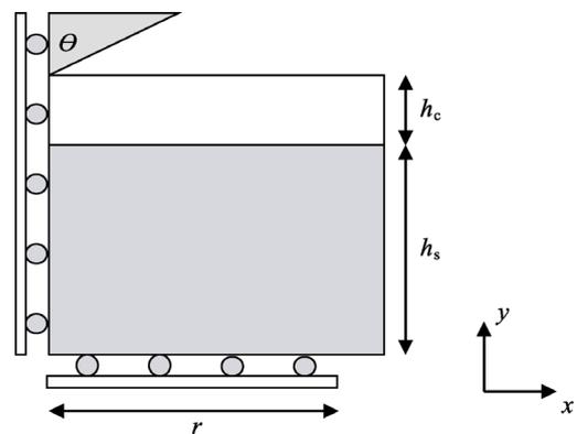
Fig. 5 Schematic of the 2D axisymmetric FEM model.
