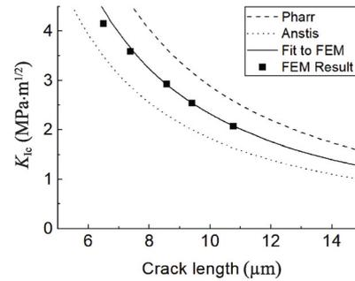
Fig. 17 Fracture toughness as a function of the length of a crack generated by instrumented indentation for different fitting constants (Jang and Pharr 0.025, Anstis *et al.* 0.016, this study).
