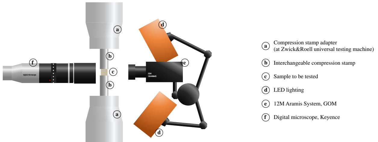
Figure 1 In-situ testing setup: Zwick&Roell universal testing machine, GOM ARAMIS Adjustable 12M System and Keyence digital microscopy [1].
