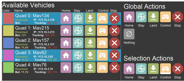
Fig. 1. Graphical user interface of the tablet application: On the left side is a list of all available UAVs with their status information. For each UAV, the color, battery level, status of the position determination and IP and MavLink address are displayed.
