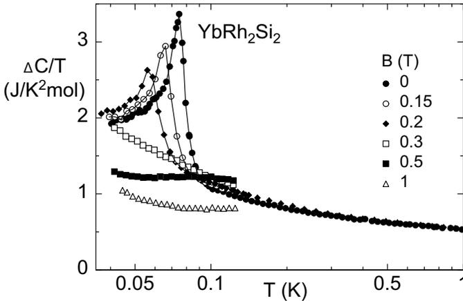
Fig. 6. Specific heat as  $\Delta C/T = (C - C_Q)/T$  vs  $T$  (on a logarithmic scale) for  $\text{YbRh}_2\text{Si}_2$  at varying fields applied parallel to the  $c$ -axis.  $C_Q \sim T^{-2}$  is the nuclear quadrupole contribution calculated from recent Mössbauer results [14].
