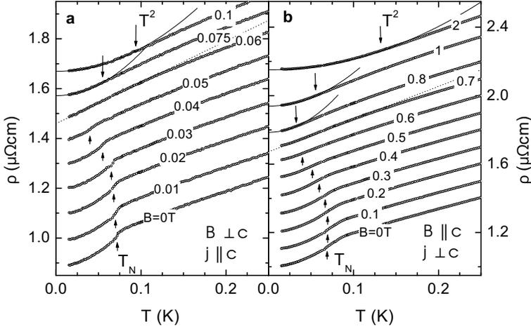
Fig. 4. Low-temperature electrical resistivity of  $\text{YbRh}_2\text{Si}_2$  at varying magnetic fields applied perpendicular (a) and along the  $c$ -axis (b). For clarity the different curves in  $B > 0$  were shifted subsequently by  $0.1 \mu\Omega\text{cm}$ . Up- and down-raising arrows indicate  $T_N$  and upper limit of  $T^2$  behavior, respectively. Dotted and solid lines represent  $\Delta\rho \sim T^\varepsilon$  with  $\varepsilon = 1$  and  $\varepsilon = 2$ , respectively.
