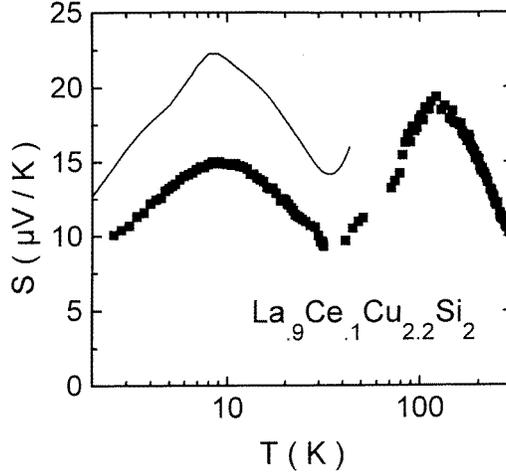
**Figure 1.** Measured thermoelectric power of  $\text{La}_{0.9}\text{Ce}_{0.1}\text{Cu}_{2.2}\text{Si}_2$  (squares) and the 4f-derived part as calculated via Gorter–Nordheim analysis (line) for  $2.5 \text{ K} < T < 300 \text{ K}$ . The low- $T$  peak is consistent with a one-channel Kondo effect of the spin-degenerate CF ground-state doublet, while the high- $T$  peak reflects excited CF levels.
