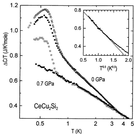
**Figure 2.**  $\Delta C/T$  versus  $T$  (on a logarithmic scale) for a polycrystalline (A-type)  $\text{CeCu}_2\text{Si}_2$  sample for  $p = 0$  and  $0.7$  GPa,  $B = 0$  (open symbols) and  $2$  T (closed symbols). The  $p = 0$  data display the A-phase transition; the  $p = 0.7$  GPa ( $B = 0$  T) data display the superconducting transition. The inset shows the  $p = 0.7$  GPa ( $B = 2$  T) data as  $\Delta C/T$  versus  $T^{1/2}$ .
