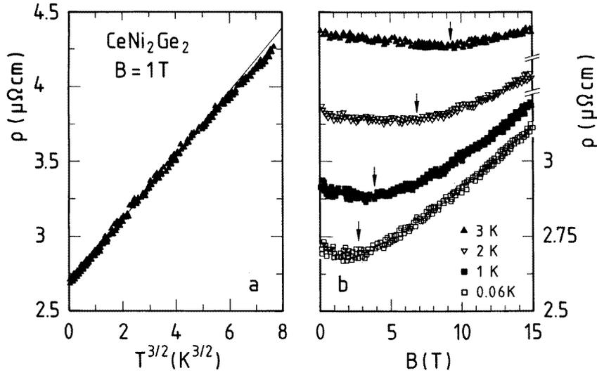
**Figure 8.** The resistivity of a polycrystalline  $\text{CeNi}_2\text{Ge}_2$  sample. (a)  $\rho$  versus  $T^{3/2}$  at  $B = 1$  T. The line represents  $\rho = \rho_0 + \beta T^{3/2}$ . (b)  $\rho$  versus  $B$  at differing temperatures. The arrows mark changes from negative to positive magnetoresistivity; see the text.
