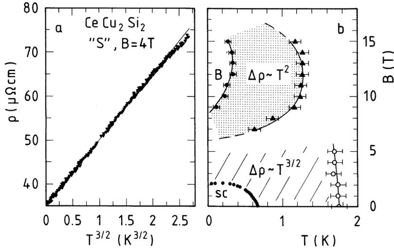
**Figure 6.** (a) The resistivity of the same single crystal as in figure 5 at  $B = 4$  T, parallel to the  $a$ -axis, i.e. longitudinal to the current. (b) The  $B$ - $T$  diagram displaying the superconducting (sc) phase and the B phase as well as ranges in which the resistivity shows ‘FL’ ( $\Delta\rho \sim T^2$ ) and ‘NFL’ ( $\Delta\rho \sim T^{3/2}$ ) behaviour, respectively.
