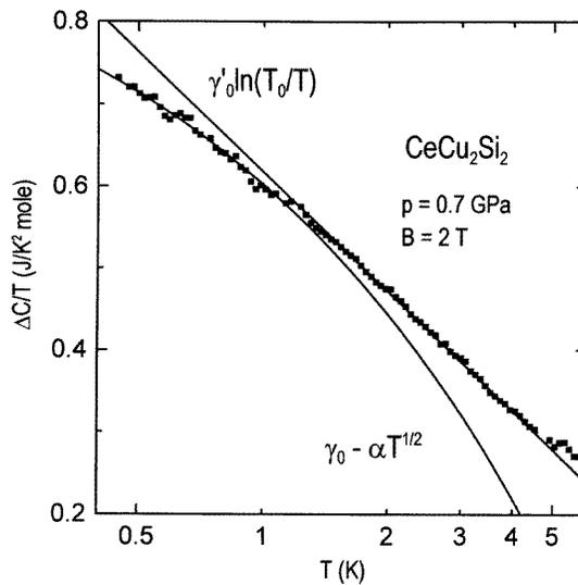
**Figure 4.**  $\Delta C/T$  versus  $T$  (on a logarithmic scale) for the same sample as in figure 2 at  $p = 0.7$  GPa and  $B = 2$  T. Lines indicate 'asymptotic' and 'crossover' temperature dependences; see the text.
