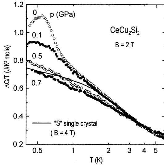
**Figure 3.**  $\Delta C/T$  versus  $T$  (on a logarithmic scale) at  $B = 2$  T and differing pressures for the same  $\text{CeCu}_2\text{Si}_2$  sample as in figure 2.  $B = 4$  T ( $p = 0$ ) results for S-type single crystal (cf. figure 5) are also shown.
