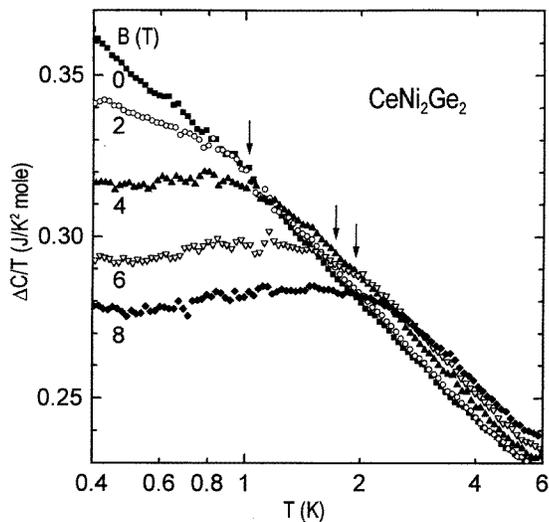
**Figure 10.** The field dependence of  $\Delta C/T$  versus  $T$  (on a logarithmic scale) for the same sample as in figure 7. The arrows mark the onset of the low- $T$  ‘FL’ regime for  $B = 4, 6$  and  $8$  T, respectively (from figure 9(a)).
