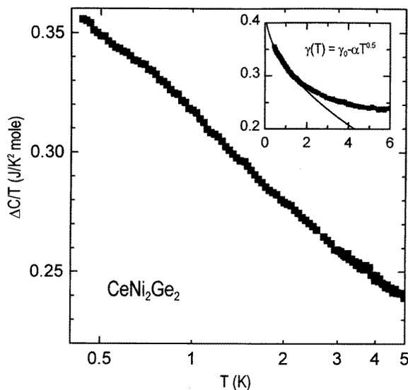
**Figure 7.**  $\Delta C/T$  versus  $T$  (on a logarithmic scale) for a polycrystalline  $\text{CeNi}_2\text{Ge}_2$  sample. Inset: the same data on a linear temperature scale. The solid line represents  $\Delta C/T = \gamma_0 - \alpha T^{1/2}$ ; see the text.
