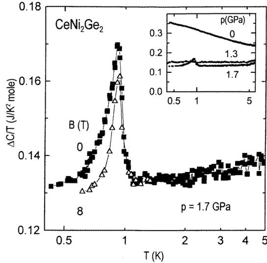
**Figure 11.** The pressure dependence of  $\Delta C/T$  versus  $T$  (on a logarithmic scale) for the same sample as in figure 7.  $B = 0$  data for differing pressure values are shown in the inset. The  $p = 1.7$  GPa data at  $B = 0$  and  $B = 8$  T indicate a non-superconducting second-order phase transition at  $T_1 = 1$  K; see the text.
