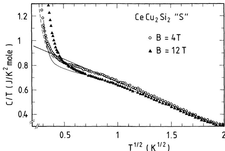
**Figure 5.** Normal-state specific heat of S-type CeCu<sub>2</sub>Si<sub>2</sub> single crystal as  $C/T$  versus  $T^{1/2}$  for two different magnetic fields applied parallel to the  $a$ -axis. Dashed ( $B = 4$  T) and thin solid ( $B = 12$  T) lines represent data after subtraction of nuclear contributions due to the external field. The thick solid line representing  $C/T = \gamma_0 - \alpha T^{1/2}$  is intended as a guide to the eye.
