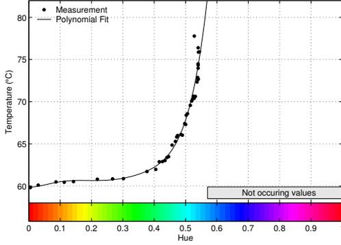
Fig. 2. TLC calibration by means of a sixth order polynomial fit to measured results. It is used for post-processing of self-heating measurements by LCT.
