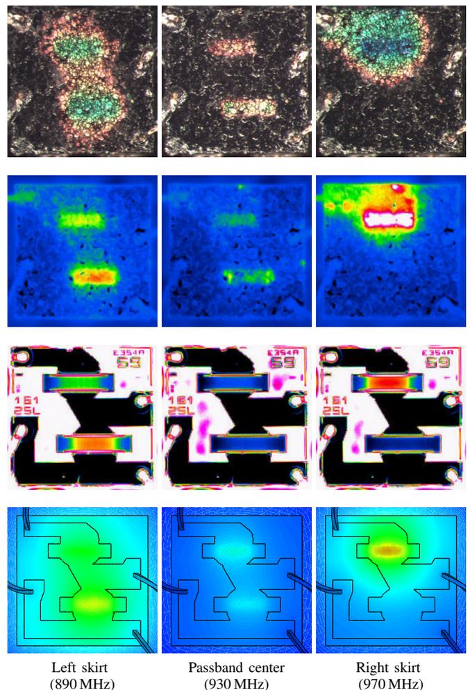
Fig. 4. Qualitative temperature distributions on a half-section ladder-type SAW filter with thick  $\text{SiO}_2$  coating under load ( $P = 25$  dBm): Measured by LCT (top panel), measured by IRT with (second panel) and without (third panel) black backing paint, and simulated using FEM (bottom panel). All are shown for three different load frequencies, at about the left skirt, at the passband center, and near to the right skirt of the filter.
