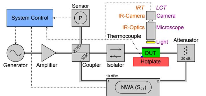
Fig. 3. Experimental setup for self-heating measurements by LCT and IRT.
