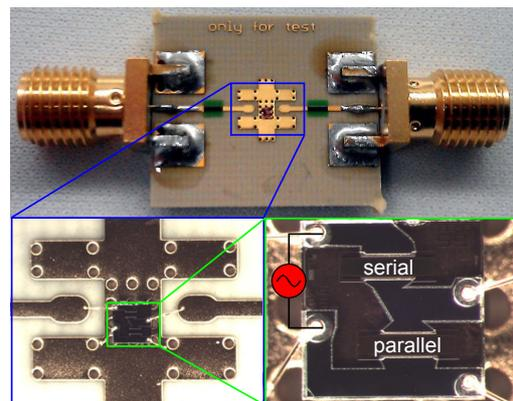
Fig. 1. The investigated device is a half-section ladder-type SAW filter consisting of one serial and one parallel resonator with the former next to the input. It is passivated with a thick SiO<sub>2</sub> coating and mounted on a PCB by an epoxy adhesive.
