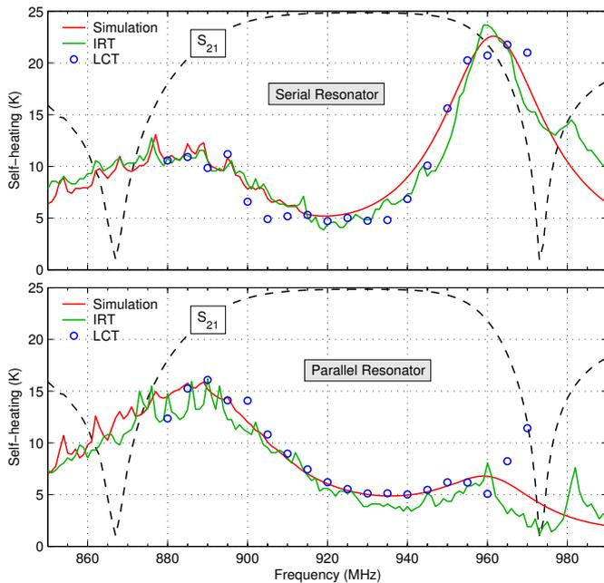
Fig. 5. Self-heating of both resonators as a function of load frequency at a load power of  $P = 25$  dBm: Simulation compared with IRT and LCT measurement results. The transfer function  $S_{21}$  of the filter is shown as a reference in arbitrary units.
