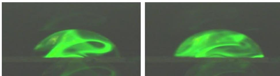
**Figure 2.** SAW induced internal streaming in a small water droplet (side view, approx. 50 nL). A dried fluorescent dye on the surface of the chip is dissolved by SAW agitation, and rapidly fills the whole droplet volume.
