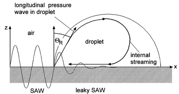
**Figure 1.** Sketch of the acoustic streaming acting on a small droplet on the surface of a piezoelectric substrate. The acoustic energy is radiated into the fluid under an angle  $\Theta_R$ , leading to internal streaming in the small fluid volume.
