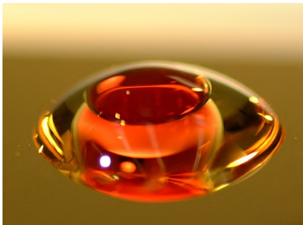
Figure 6. ‘Virtual liquid test tube’ for high temperature application of the planar SAW driven fluidics. To avoid evaporation of the aqueous sample solution (red), the droplet has been covered by a thin mineral oil layer. Both represent a fluid test tube for further processing of the sample.
