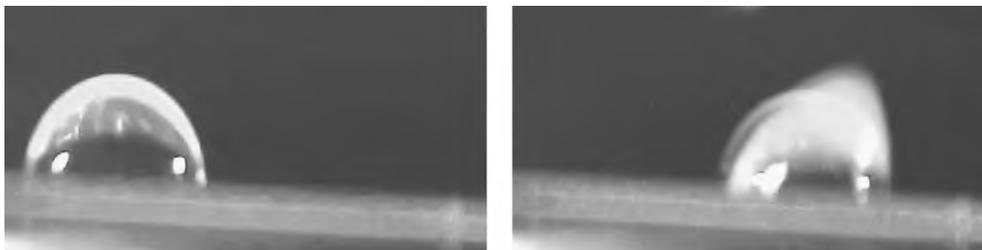
**Figure 4.** Side view of a small droplet (ca. 50 nL) on the surface of a piezoelectric substrate. Left: droplet in rest, note the wetting angle of about 90°, which has been obtained by a hydrophobic treatment of the surface. Right: droplet being “hit” by a SAW impinging from the left. The acoustic radiation strongly deforms the droplet shape. This leads to a momentary asymmetry of the wetting angles of the droplet.
