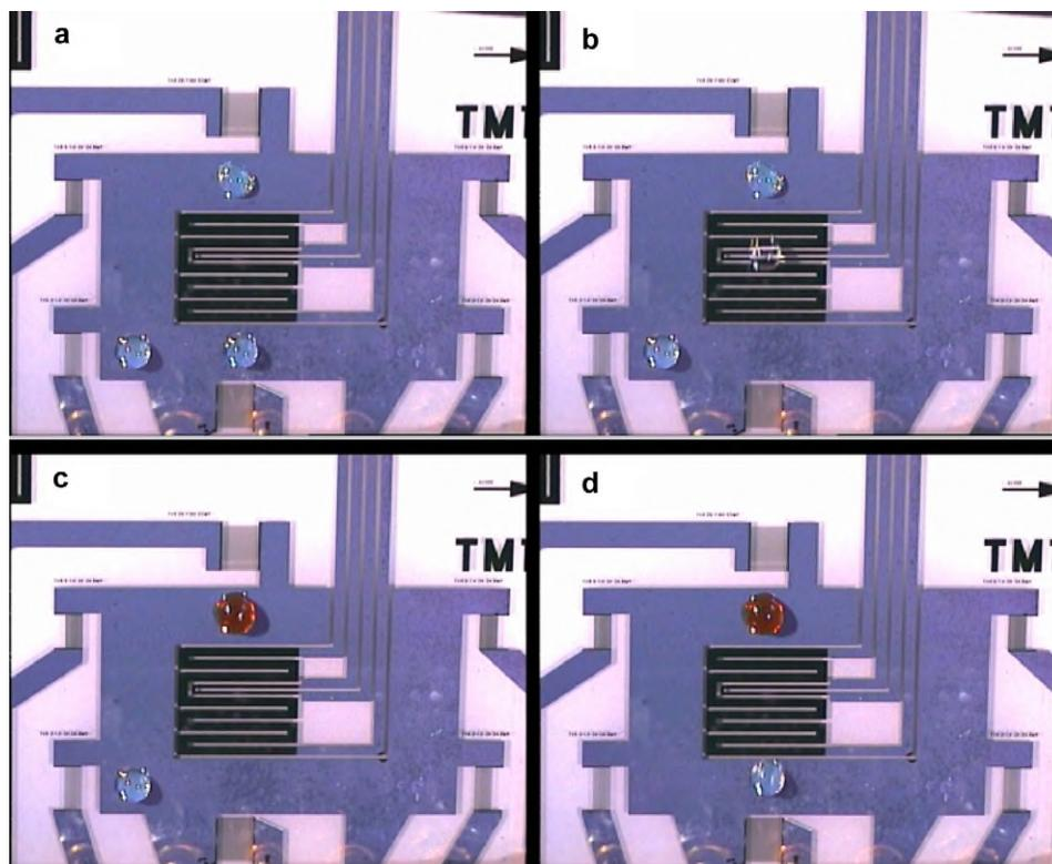
**Figure 5.** A SAW driven microfluidic processor. Three droplets (approx. 100 nL each) are moved ‘remotely controlled’ and independently by the nanopumps. (a)–(d) represent a series of subsequently taken snapshots to visualize the movement, and the ‘nanochemical reactions’ occurring when the droplets are merged and mixed by the action of the surface wave. The chip not only contains the nanopumps and the fluidic environment, but also the center additional real estate like sensors and heaters.
