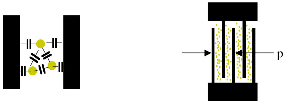
Fig. 2: Schematic sketch of an electrode structure for determination of the RF impedance within a hybridization spot. The surface bound gold beads couple primarily capacitively to the electrodes. Hence, the RF impedance of the latter depends on the degree of the gold coating upon the active area. p depicts the finger periodicity of the electrode structure.
