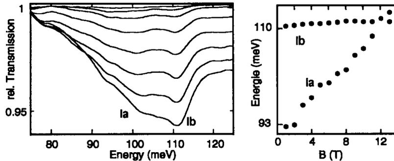
Fig. 2. The spin-flip resonances can be clearly resolved at low magnetic fields ( $B \leq 8$  T with  $\Delta B = 1$  T). Transition Ib is roughly constant in energy and has a greater oscillator strength (area under the curve) than transition Ia. Line Ia, on the other hand, shifts to higher energies as the magnetic field is increased.
