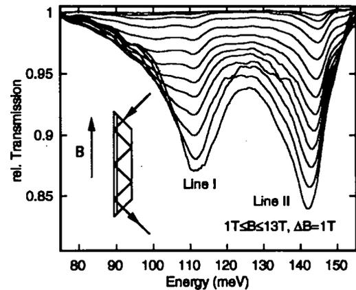
Fig. 1. Relative transmission spectra for  $B \leq 13$  T with  $\Delta B = 1$  T in the multiple reflection path geometry (inset). At high magnetic fields two resonances (I and II) can be seen which both gain oscillator strength as the field is increased. At low fields resonance I splits into two lines, giving experimental evidence for a zero-field spin-splitting.
