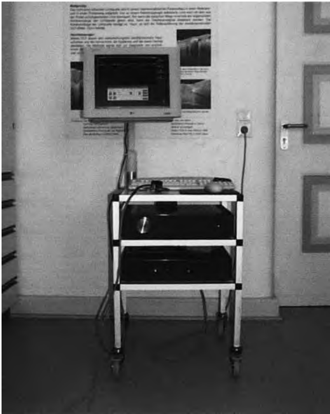
Fig. 3. The OCT system and the hand piece in front of the keyboard.
