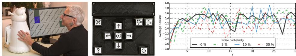
**Figure 1.5** Left: a study participant interacts with an adaptive social robot in Ritschel et al. [2019d]. Middle: the hardware control panel is used for interaction and to give a reward signal for reinforcement learning (adapted from Ritschel et al. [2019d]). Right: simulation results of a robot with adaptive extraversion in Ritschel et al. [2017]. Reeti robot by Robopec.
