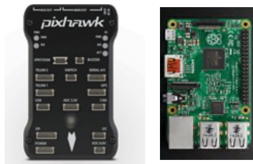
Figure 3. The pixhawk autopilot system (left) and the Raspberry acquisition board (right).
