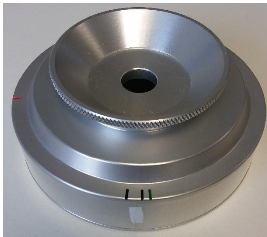
Figure 7: drum of a Hirst-type pollen sampler with Melinex ® tape (photo by Franziska Kolek)
