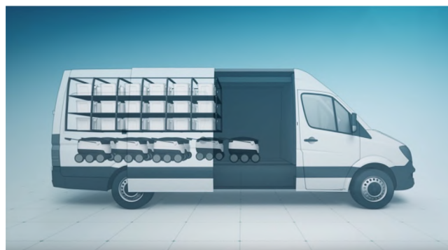
Fig. 1. Specialized truck with freight containers and delivery robots (Mercedes-Benz Vans, 2016).
