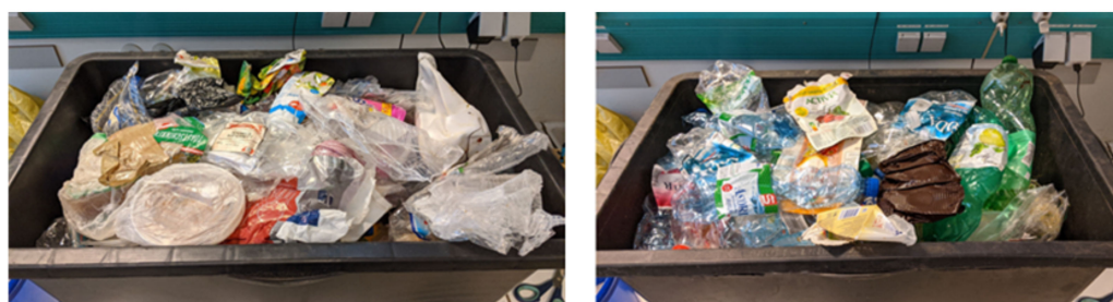
Figure 1. Exemplary manually pre-sorted bulky three-dimensional plastic packaging waste. Left: Two-dimensional flexible plastic waste. Right: Three-dimensional solid plastic waste.
