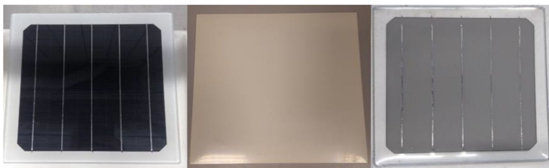
Figure 2. Module samples: frontside (left), backside without pre-treatment (middle), backside with pre-treatment (right).
