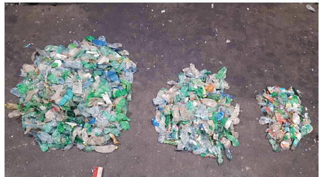
FIGURE 3: Output fraction of the delabeller - from left to right: category 1 (Good), category 2 (Middle), category 3 (Bad).
