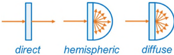
Figure 3. Measurement of direct, hemispheric and diffuse transmittance.
