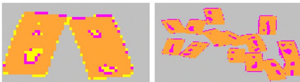
Figure 8. Misclassification of object pixels owing to water drops on TPU particles (orange): PP (pink) and unknown (yellow).
