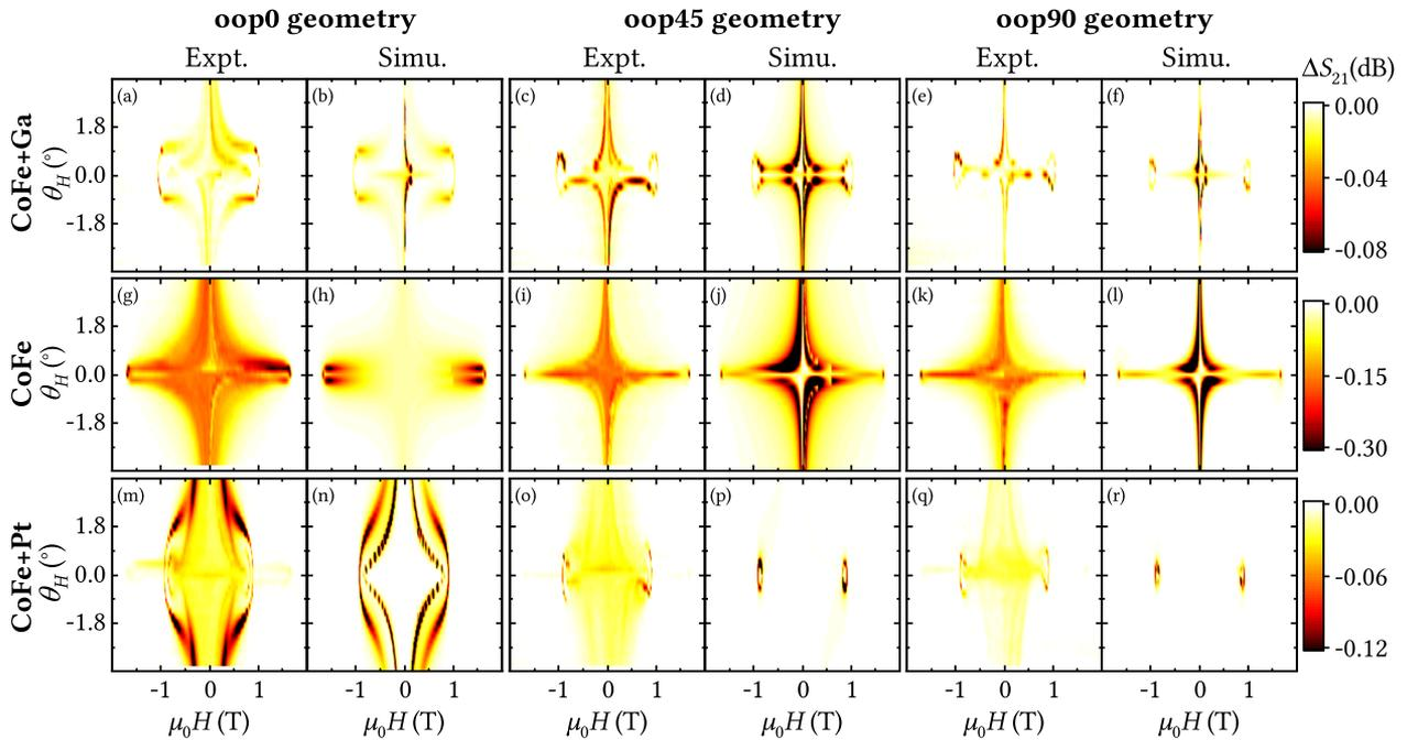
**FIG. 8.** The magnetoacoustic transmission  $\Delta S_{21}(\mu_0 H, \theta_H)$  of the magnetic micro-strips CoFe + Ga (2.78 GHz), CoFe (2.96 GHz), and CoFe + Pt (3.17 GHz) is shown in the oop0-, oop45-, and oop90-geometry (see Fig. 3) for almost out-of-plane oriented external magnetic field ( $\theta_H = -3.6^\circ, \dots, 3.6^\circ$ ). Simulation and experiment show good qualitative agreement.
