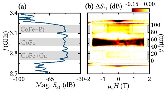
**FIG. 6.** (a) The transmission characteristics of the fabricated device shows the expected wide band behavior. (b) Within this transmission band, the magnetoacoustic transmission  $\Delta S_{21}(\mu_0 H)$  differs for the three different frequency sub-bands that correspond to the three different magnetic films.
