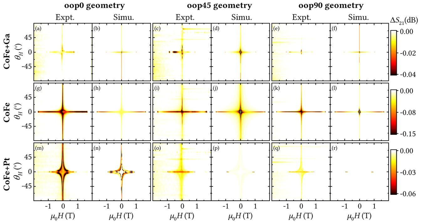
**FIG. 7.** The magnetoacoustic transmission  $\Delta S_{21}(\mu_0 H, \theta_H)$  of the magnetic micro-strips CoFe + Ga (2.78 GHz), CoFe (2.96 GHz), and CoFe + Pt (3.17 GHz) is shown in the oop0-, oop45-, and oop90-geometry (see Fig. 3). Resonances are observed for  $\theta_H = 0^\circ$ , which are studied in more detail in Fig. 8. Simulation and experiment show good qualitative agreement.
