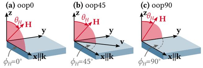
**FIG. 3.** The magnetoacoustic transmission is studied in the three geometries oop0, oop45, and oop90, which are defined by the polar angle  $\phi_H$  of the external magnetic field  $\mathbf{H}$ . Here,  $\mathbf{H}$  is tilted with respect to the  $z$  axis by the azimuthal angle  $\theta_H$ .
