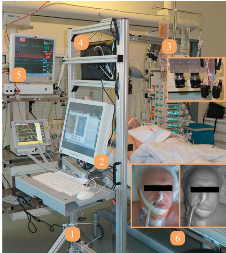
Fig. 1. cbPPG Measuring System: 1 – construction set-up, 2 – recording PC, 3 – sensing system with RGB and NIR camera (left) and NIR light source (right), 4 – additional display, 5 – GE patient monitor, 6 – video recording area (left: RGB, right: NIR).
